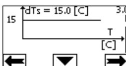
In this case the circulator increases or decreases the flow rate to keep the absolute difference between T and T1 constant at dTs = 15°C.
