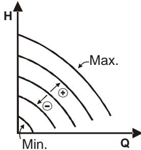
The rotation speed is kept at a constant number of revolutions. This rotation speed may be set between a minimum value and the rated frequency of the circulation pump (e.g. between 15 Hz and 50 Hz).
