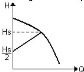
In this adjustment mode the differential pressure is reduced or increased as the water request falls or rises.
