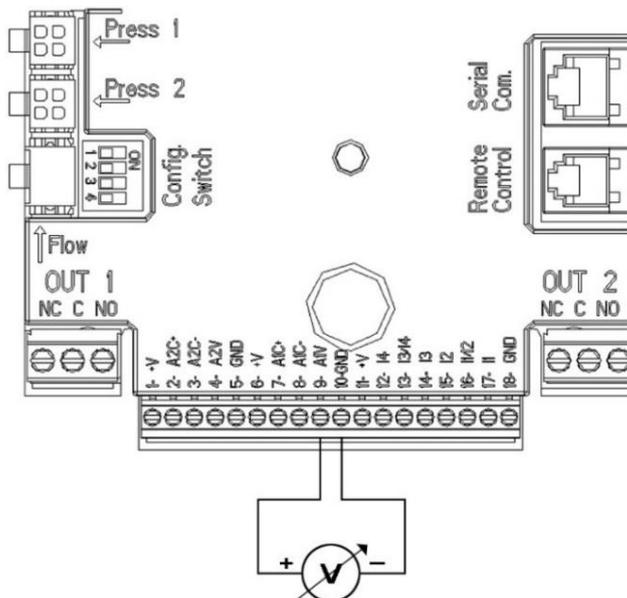
Figure 6: Example of Connection of Analogue Input
