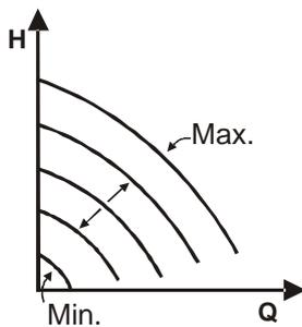
The rotation speed is kept at a constant number of revolutions in proportion to the voltage of the external analogue signal (see par. 5.5.2). The rotation speed varies in linear mode between the rated frequency of the pump when  $V_{in} = 10V$  and the minimum frequency when  $V_{in} = 0V$ .
