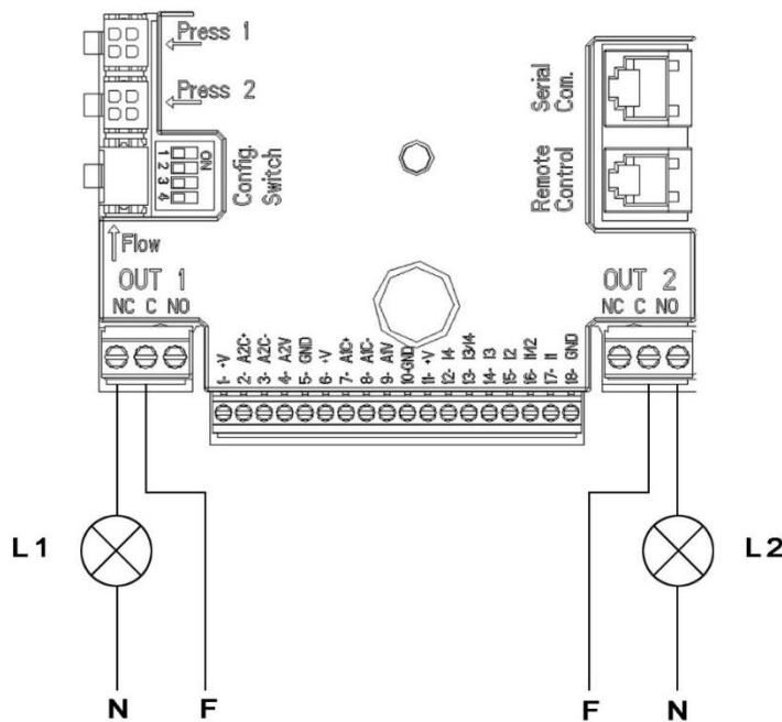
Figure 9: Example of Connection of Digital Outputs
