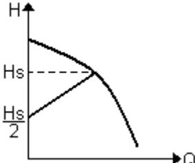
In this adjustment mode the differential pressure is reduced or increased as the water request falls or rises.
