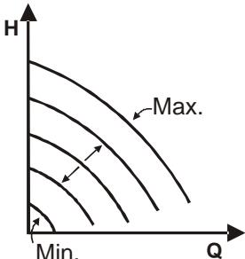
The rotation speed is kept at a constant number of revolutions in proportion to the voltage of the external analogue signal (see par. 5.5.2). The rotation speed varies in linear mode between the rated frequency of the pump when  $V_{in} = 10V$  and the minimum frequency when  $V_{in} = 0V$ .
