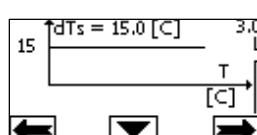
In this case the circulator increases or decreases the flow rate to keep the absolute difference between  $T$  and  $T1$  constant at  $dTs = 15^\circ\text{C}$ .
