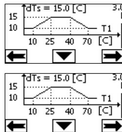
$$1) \text{ Av } T1 \leq 10^{\circ}\text{C} \Rightarrow dTs = |T-T1| = 10^{\circ}\text{C}$$
