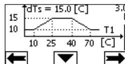
1) Si  $T1 \leq 10^{\circ}\text{C} \Rightarrow dTs = |T-T1| = 10^{\circ}\text{C}$
